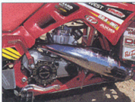
Desert racing goes high-tech! The combination of the Paul Turner pipe and PC 2000 cylinder with power valve (seen just above the exhaust manifold) produces smooth, strong power.
