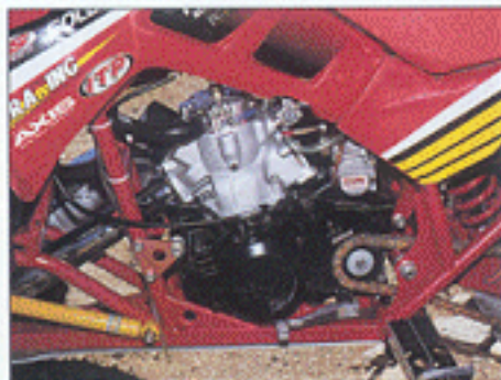
A 37mm Keihin carb gets the air flowing into both desert quads. Check out the double footpegs for more support. Though this machine has a Bilstein steering stabilizer (just below the left front motor mount), the team plans to use GPR stabilizers on both machines. They are adjustable on the fly and fully rebuildable.
