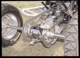
Check out that burly, four-piston rear brake caliper, which is from a Yamaha FJ1200 motorcycle. The pad used in it lasts the entire 12 hours.
