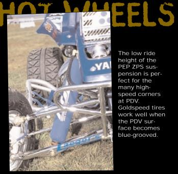
The low ride height of the PEP ZPS suspension is perfect for the many highspeed corners at PDV. Goldspeed tires work well when the PDV surface becomes blue-grooved.
