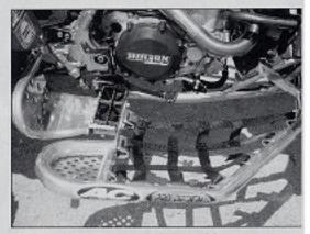
Chromed AC Rading nerf bars with IMS/Roll Design extra wide fcotpegs and lender guards help keep the rider's feet planted solidly on the Duncan YFZ450. A Hinson Racing clutch helps keep the motor hooking up under the extreme demands of a top pro rider
