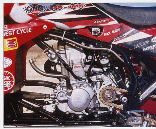
To make it easier to add oil, the GWC quad has a long filler tube attached to the oil cap. TRX450R owners have to remember to check and change the oil on both sides of this engine.
