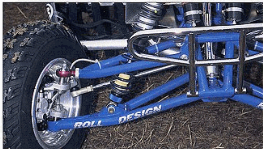
Up front, Lohr's machine features the Lobo gull wing A-arm design. Custom Axis shocks and Holeshoot MX tires are found front and rear.
