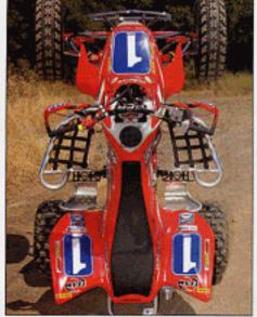
The IMS Dry Break tank holds a full four gallons for good range between pits stops. The combination of TAG aluminum bars and GPR stabilizer kept our hands and arms fresh, despite the extreme terrain.
