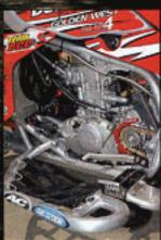
Not much was done on the bottom end of the 450R's motor, but the top end was completely reworked, from the valve springs down to the displacement- and compression-enhancing DRIJE piston. The Edelbrock carb eliminates the need for a hot start button.
