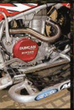
Duncon Racing and Hinson Racing teamed up to make a beefier clutch to handle the extra power of the modified 450R motor. It doesn't slip and it's not stiff. The extra-wide IMS pegs provide a great platform, especially when landing from jumps or hammering through brutal terrain.
