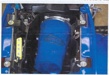
**Step 3:** Remove the Vortex ECU from its package and slide into the Vortex rubber mounting boot. Slot the ECU and Mounting boot onto the stainless mounting bracket provided and bolt onto the side of the airbox.
