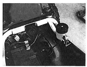
Step 2: Mount the EFI Interceptor in behind the tool tray under the seat. Use the Velcro provided to secure it in place. Note: Always clean the plastic surface with alcohol before applying the Velcro. Step 3: Route the main wiring harness down the right hand side of the frame towards the right side of the throttle body.
