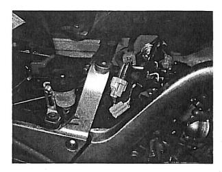
**Step 8:** Plug in the Grey 3 Way connector from the EFI Interceptor harness into the Black 3 way connector previously unplugged from the Throttle Position Sensor.
