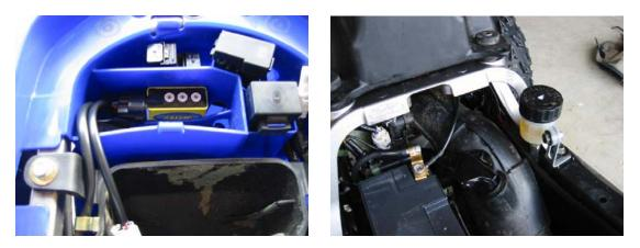
**Step 2:** Mount the EFI Interceptor in behind the tool tray under the seat. Use the Velcro provided to secure it in place. Note: Always clean the plastic surface with alcohol before applying the Velcro. **Step 3:** Route the main wiring harness down the right hand side of the frame towards the right side of the throttle body.
