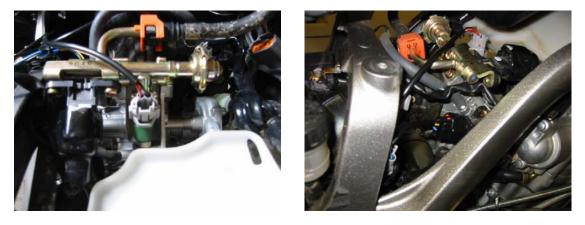
**Step 5:** Lift the petrol tank to one side and unplug the grey 2 Way Fuel Injector connector. Plug the Blue 2way connector from the EFI Interceptor into this connector.
