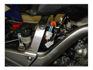
Step 8: Plug in the Grey 3 Way connector from the EFI Interceptor harness into the Black 3 way connector previously unplugged from the Throttle Position Sensor.Step 9: Use the zip ties provided to secure the loose wiring. Replace the petrol tank, battery bracket, rubber cover, front plastic shroud and seat. Installation of the EFI Interceptor is now complete!
