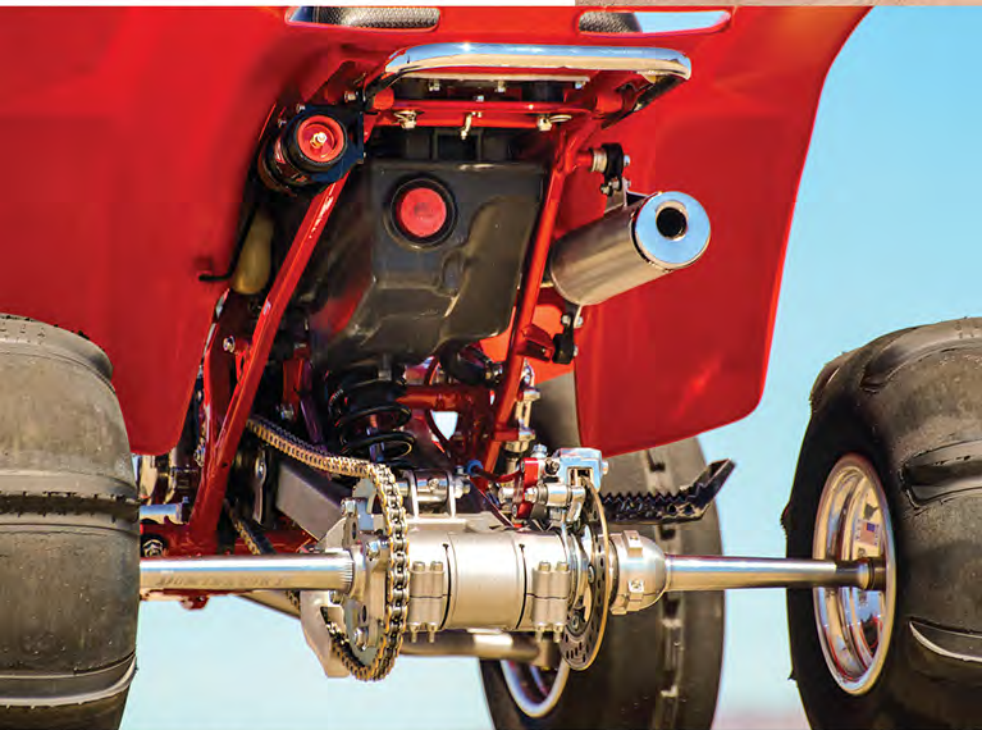
A Laeger's +1 swingarm keeps the 300's ample power from producing unwanted wheelies and adds stability for high-speed straights.
