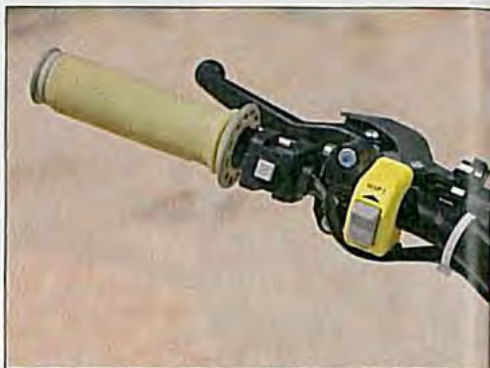
A clean start button and ignition-map switch for the Dynatek ignition box take the place of the clunky light pod on the stock bars.
