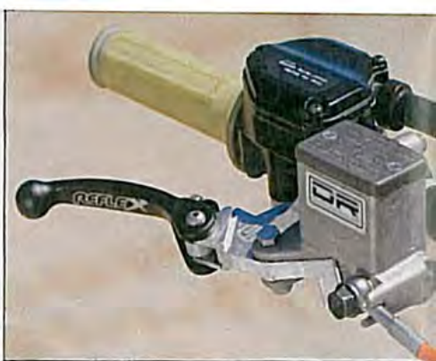
Sunline Reflex folding levers and Renthal Kevlar grips adorn the Renthal Fatbars, which make the ergonomics of the Honda much better.
