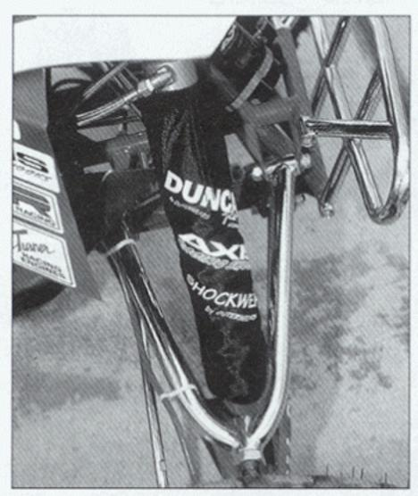
Custom Axis shocks offer 10.75 inches of travel up front on the LOBO chassis. Roll believes in running suspension that employs a lot of sag to keep the machine's center of gravity lower without sacrificing travel.
