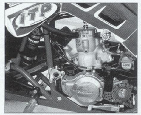
In the motor department, Duncan Racing installed one of their PC2000 Power valve cylinder kits on Spader's Honda. It uses a 265cc engine bore (legal in AMA/GNC racing), a Hinson Billet clutch basket to keep the clutch healthy, a Duncan Racing Pyramid reed valve, and Paul Turner #TS08 pipe and Fat Boy silencer.
