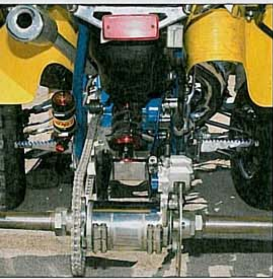
The swingarm on this big 500cc two-stroke was replaced with a 2-inch-longer unit from Leagers. Without it, the machine would flip over backwards since it has so much power.
