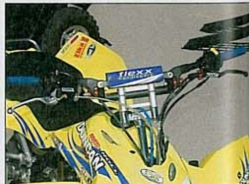
A set of Fasst Co Flexx bars mounted on both machines took care of the vibration on the two-stroke and smoothed the rigid nature of the four-stroke's chassis.
