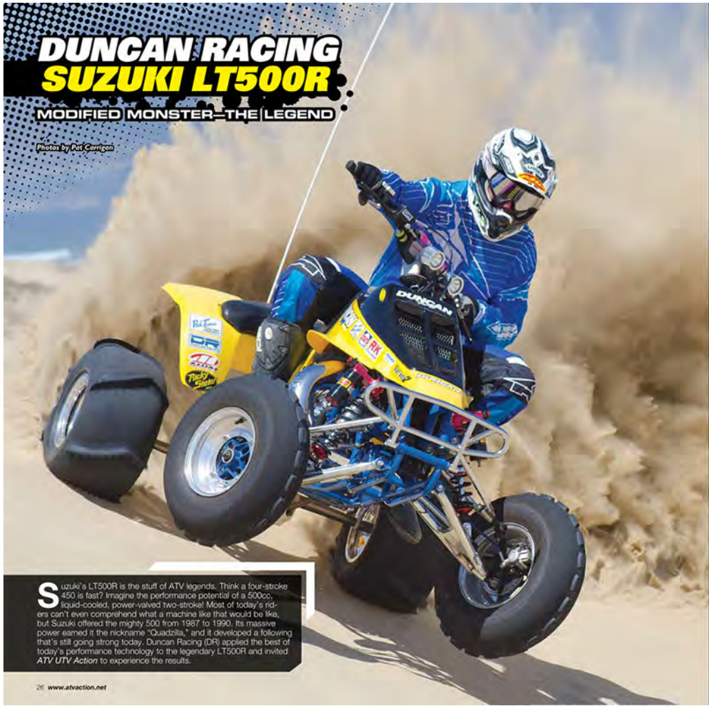
The liquid-cooled, reed-valve, power-valve, 500cc, two-stroke engine from 1990 was advanced even by modern standards. Duncan Racing's National midrange engine kit boosts the power dramatically, but it's very controllable.
