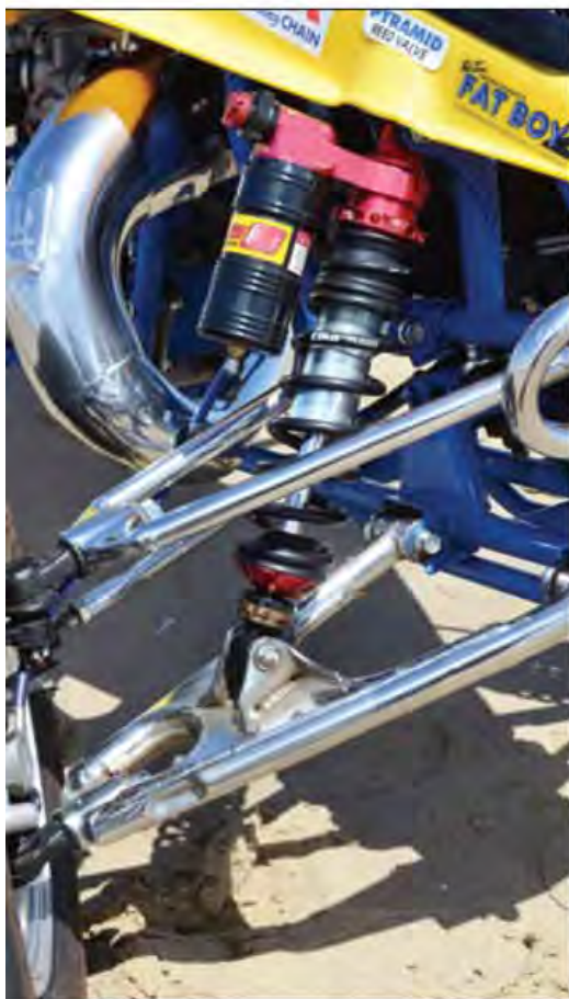
Fully adjustable Elka Stage 4 shocks bring state-of-the-art suspension to the 1990 Suzuki 500.
