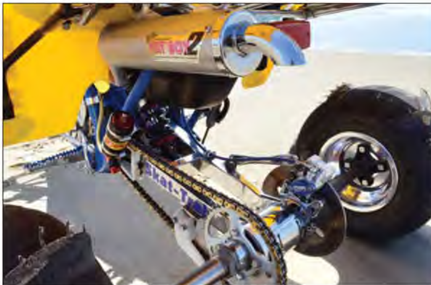
Duncan Racing has been modifying, tuning and perfecting the LT500R since it was introduced in 1987. The 2-inch-plus Laeger swingarm helps keep the 500's front end on the ground and ends the cracking problems that affect stock swingarms that have seen lots of hard use.
