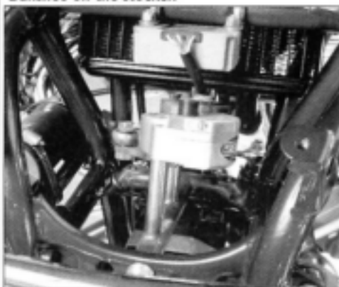
Here's one of the trickiest goodies on the Banshee. Instead of mounting the Scotts steering stabilizer on the top of the steering stem, where it can get in an argument with your face, Roll Design moved the stabilizer to the bottom of the stem. This is a custom setup, but Roll may offer it to other Banshee owners in the future.
