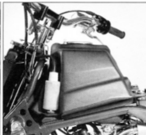
The stock tank was filled with hot water and carefully molded to accept a custom dry brake system. That cosmetics bottle at the front of the fuel tank is the radiator overflow tank, which is at the back of the Banshee on the stocker.
