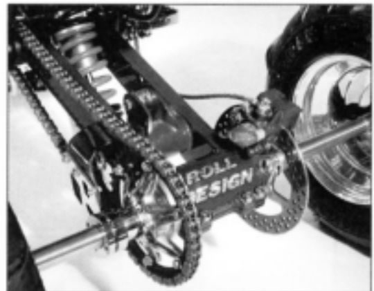
The 18.5-inch Roll swingarm retains full linkage. An RPM +4-inch Dominator axle is used for increased stability in the dunes and on the track. Wheel travel with the Custom Axis shock is a full foot!
