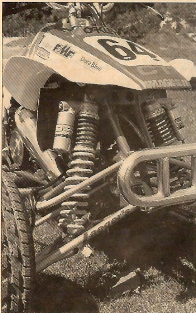
Shepherd started the contest with these massive PPS Ohlins shocks on the front end of his quad. After encountering some bottoming-out problems, he switched front shocks and cut a full second off his lap times.
