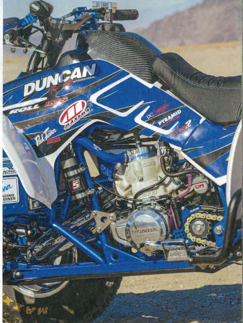
Above: Very little of the stock TRX engine remains. Aftermarket parts replace the intake, exhaust, cylinder, head, piston, clutch and gears! Left: A carbon cover hides the IMS tank. Lighting (front and rear) is from Baja Designs. That blue billet clutch perch and lever are from Beringer.
