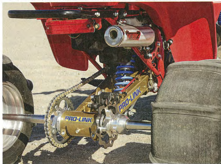
Top: This Duncan ATC is hard to get out of a turn without the front wheel in the air. The paddles were temporary. The owner ordered stock wheels and knobbies for trail use. Bottom: Duncan upgraded the ATC to a later swingarm and linkage. The axle and all associated hardware are aftermarket parts.
