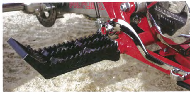
Roll Design footpegs have sharp teeth and a kick-up at the end of the peg that offers great foot traction.
